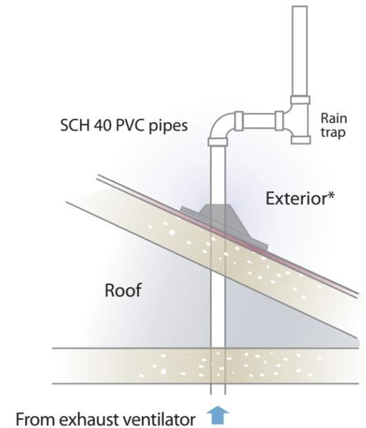
**\* Please note:** AAMI guidelines recommend that all EO sterilizers should be vented (exhausted) through a dedicated vent line to the outside atmosphere directly or through an emission control system. The vent should not terminate within 25 feet (7.6m) of any building air intake source or near pedestrian or animal traffic, nor should it allow EO release into or to reenter the building.
