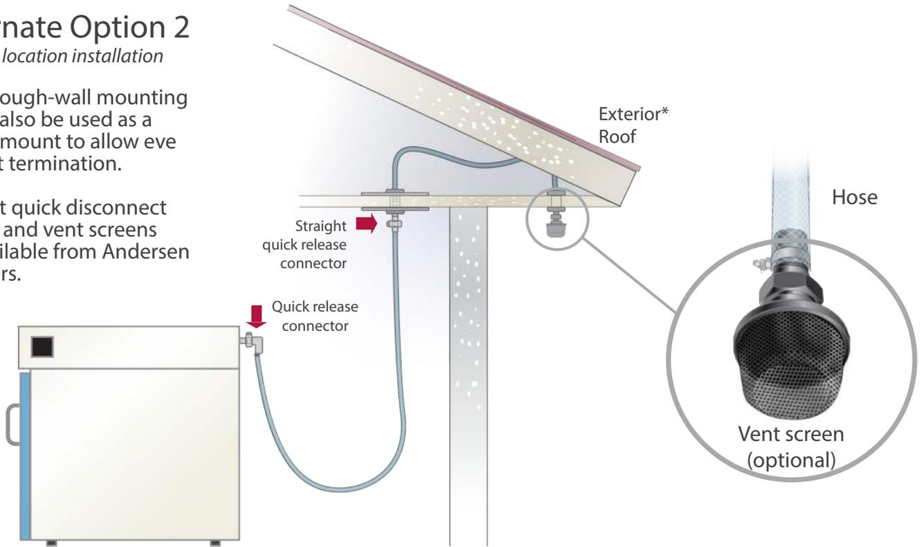
**Important:** Each EO Gas 4 Sterilizer must have its own dedicated exhaust to outside air. The exhaust streams from multiple sterilizers may not be combined into a single exhaust stream that then vents to the outside.
